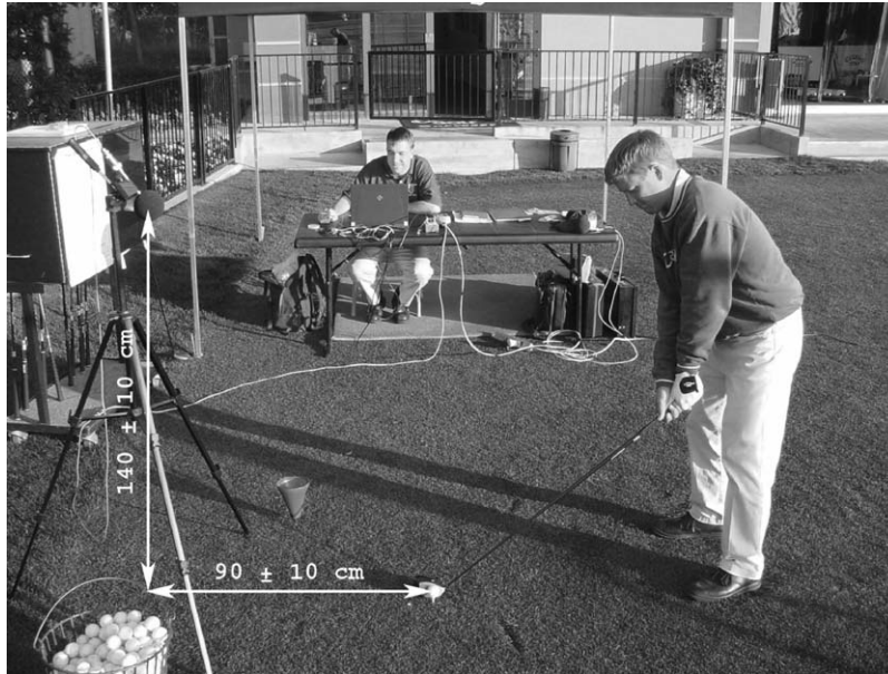
Fig. 1. Microphone location in the test set-up.
